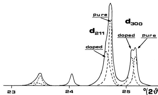
Fig. 6. Decomposed X-ray powder pattern ( $\lambda = \text{Cu K}\alpha_1$ ) of sucrose grown in the presence of *Actilight*<sup>®</sup> (0.83 g/100 g H<sub>2</sub>O), in the range  $23^\circ < 2\theta < 25.5^\circ$ . Diffraction peaks of spacing  $d_{211}$  and  $d_{300}$  show the profile splitting due to contributions of both pure and doped crystal regions.
