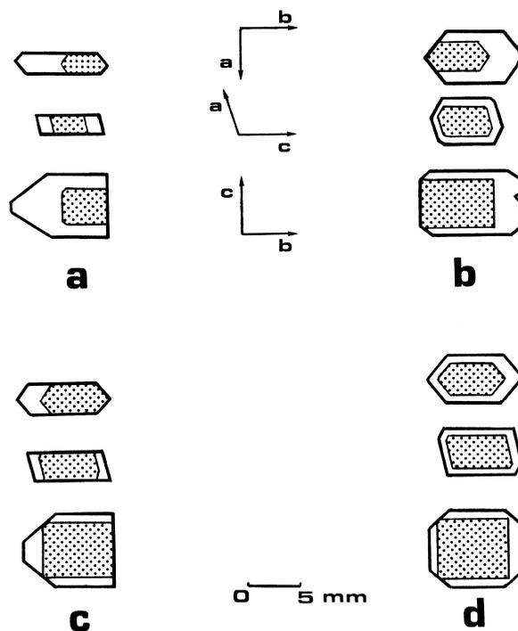
Fig. 4. Schematic drawings illustrating growth habits of sucrose crystals modified by: (a) *neo*-kestose (20 g/100 g H<sub>2</sub>O); (b) 1-kestose (20 g/100 g H<sub>2</sub>O); (c) *neo*-kestose+1-kestose (1:1); *neo*-kestose+1-kestose (1:5).
