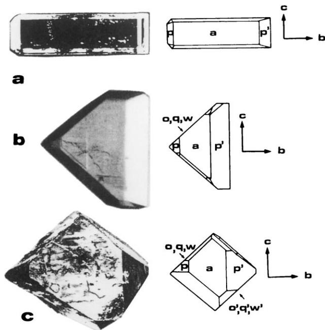
Fig. 3. Sucrose crystals grown in the presence of: (a) raffinose; (b,c) *Actilight*<sup>®</sup> (see text).
