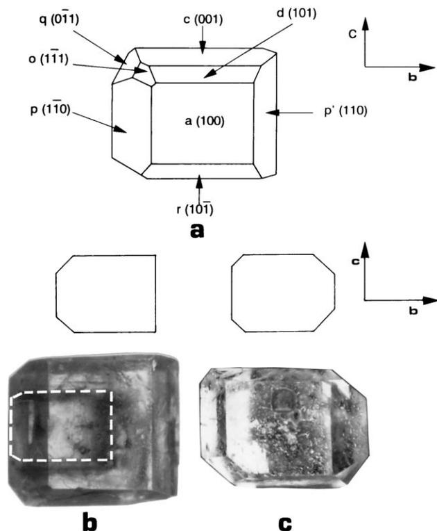
Fig. 1. Growth habits of sucrose crystals: (a) schematic drawing of the "standard" habit, showing important forms; (b) crystal grown in the presence of 150 g glucose/100 g H<sub>2</sub>O, dashed white lines define the seed —  $\{1\bar{1}0\}$  form is stopped; (c) crystal grown in the presence of 150 g fructose/100 g H<sub>2</sub>O — the habit is more symmetrical with respect to the  $(ac)$  plane, because of the slowing down of the growth rate of  $\{011\}$  and  $\{111\}$  forms.
